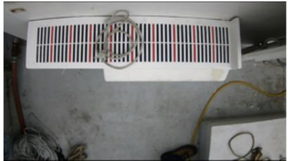
Figure 1: An example of a restricted field of view that captures only the measuring strip and its immediate surroundings. This tight view limits the amount of noise an algorithm needs to accommodate in the area surrounding the activity of interest. Image provided by the NE groundfish audit project.
