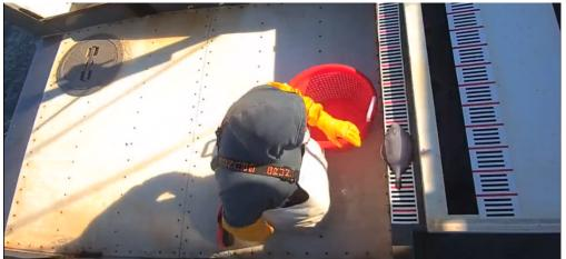
Figure 4: A fisherman measures discarded fish, using a measuring strip installed below the EM camera. The fish length, and calculated weight is captured during video review using this image. Image provided by the NE groundfish audit project.
