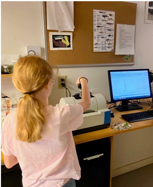
Figure 6: Putting plastic in the FTIR next to computer with the plastic graph
