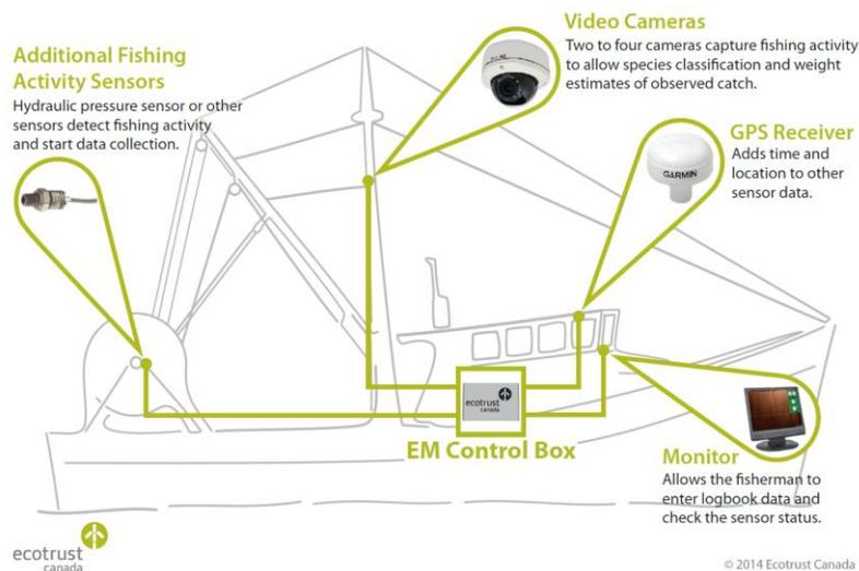
**Figure 1:** Schematic of hardware included in Ecotrust Canada's EM system
